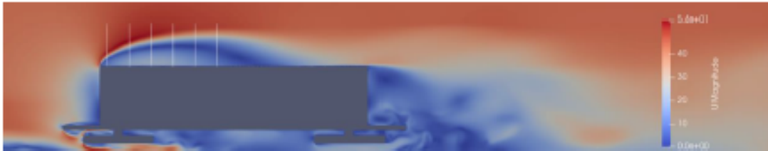
Figure 13: Magnitude velocity field of the unsteady simulation of the medium detailed geometry.
