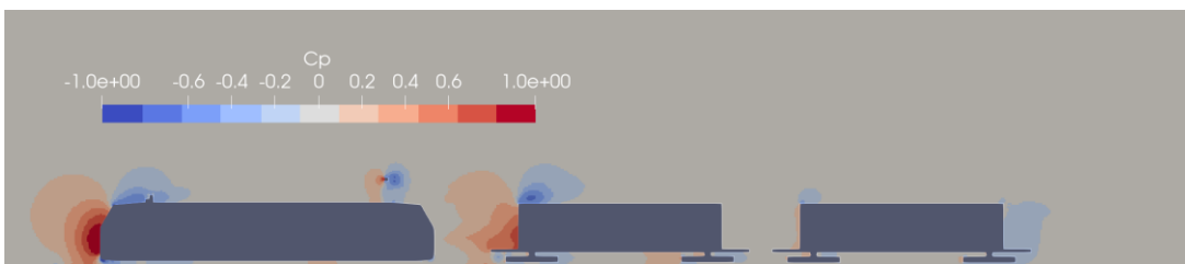
Figure 18, Time-averaged pressure coefficient field in unsteady multi-vehicle simulation
