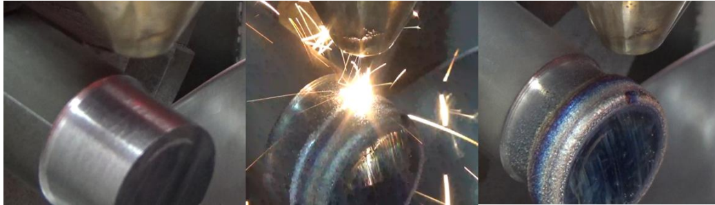
Fig. 15. Additive manufacturing of cylinder specimen by MAM (before, during, and after the MAM process)
