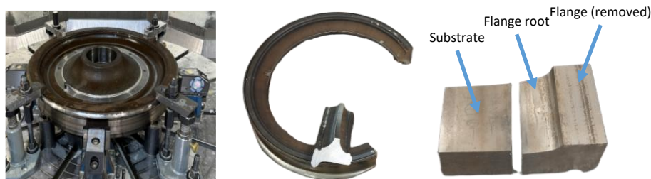
Fig. 5. Wheel machining and extraction of specimens.
